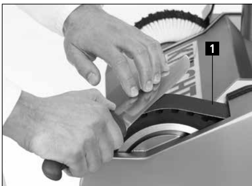
Figure 7-7 Grinding the hand knife
