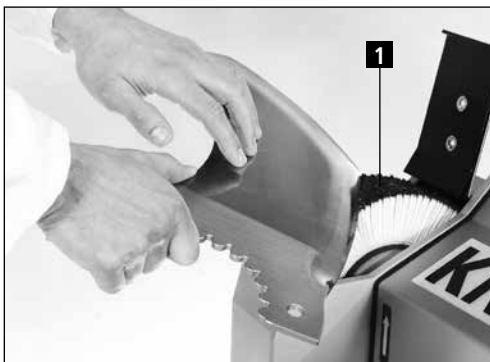
Figure 7-6 Polishing/deburring the cutter blade
