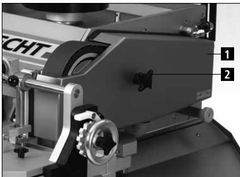
Figure 7-13 Opening the belt protective hood
