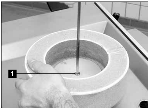
Figure 7-12 Changing the grinding disk
