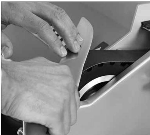
**Figure 7-2** Grinding hand knives
