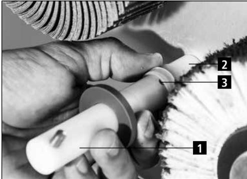
**Figure 7-16** Closing the water nozzle
