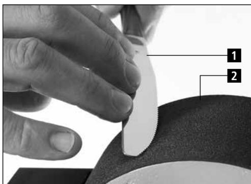
Figure 7-9 Grinding notches
