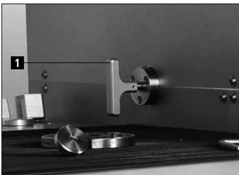
Figure 7-13 "Rotary table" stop
