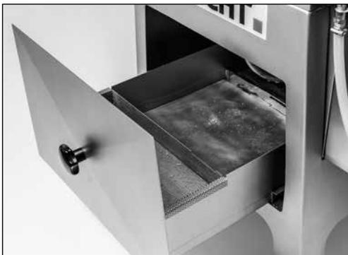
**Figure 6-1** Filling the coolant unit
