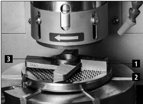
Figure 7-12 Mincing knife on rotary table
