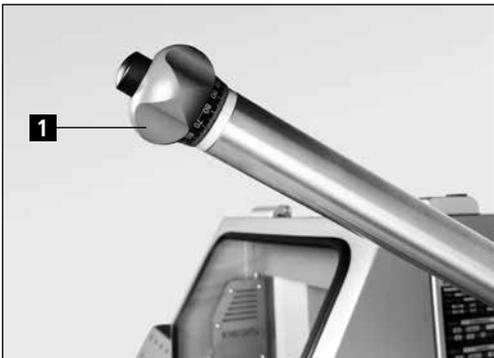
Figure 7-2 "Grinding unit" control lever
