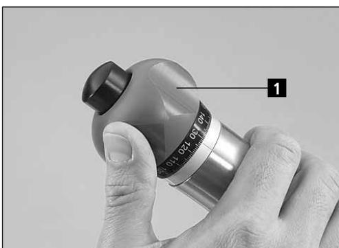
Figure 7-11 "Grinding unit" fine feed
