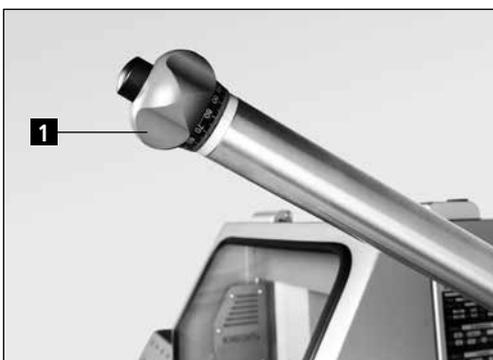
Figure 7-14 "Grinding unit" control lever
