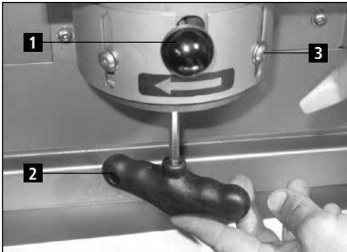
Figure 7-16 Changing the CBN grinding wheel
