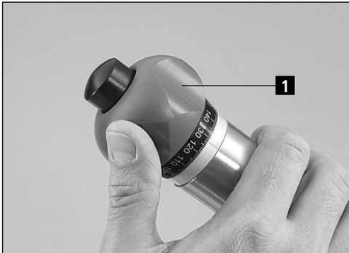
Figure 7-15 "Grinding unit" fine feed
