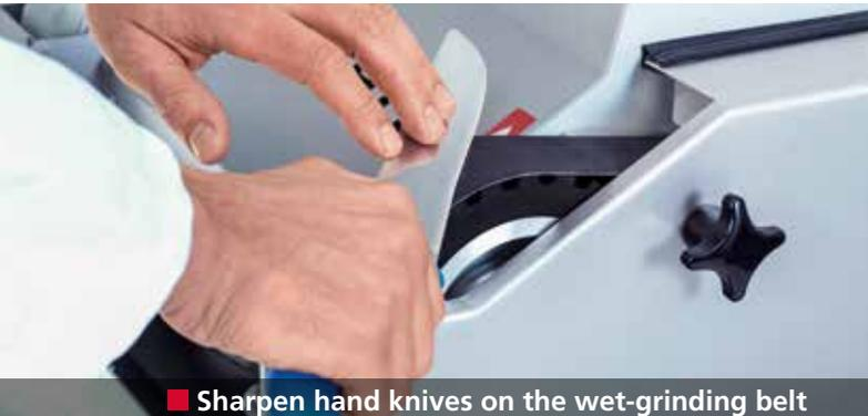
■ Sharpen hand knives on the wet-grinding belt
