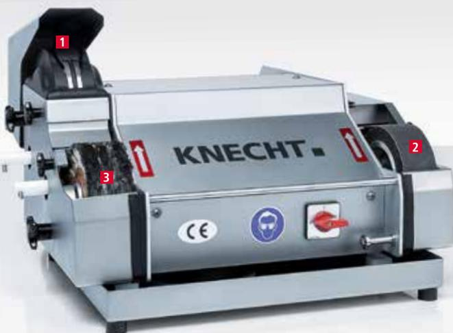
1 Hand knife grinding attachment HV 150
