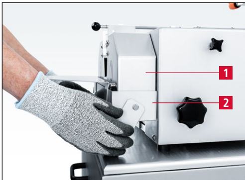
Figure 7-100 Remounting the protection hood and the water tray
