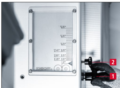
Figure 7-45 Locking the display arrow
