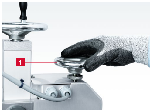
Figure 7-26 Turning the "Fine adjustment" hand wheel clockwise
