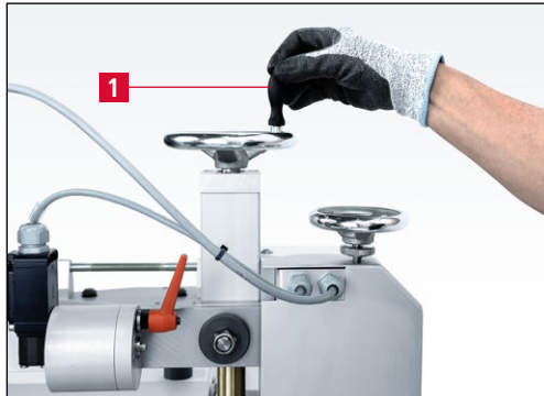
Figure 7-66 Moving the circular knife to the grinding wheels
