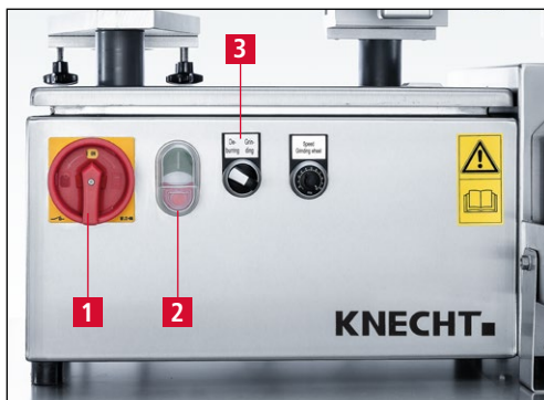
Figure 6-2 Switching on the circular knife sharpening machine
