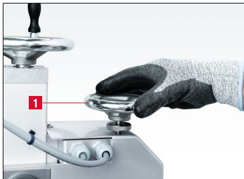
Figure 7-71 Turning the "Fine adjustment" hand wheel counterclockwise
