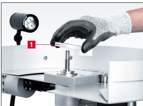
Figure 7-13 Removing clamping flange
