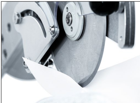
Figure 7-75 Checking the knife sharpness
