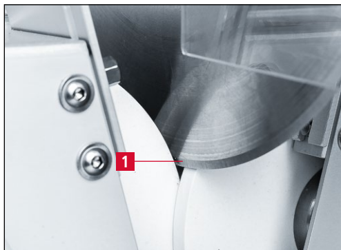
Figure 7-27 Knife moving away from the grinding wheels
