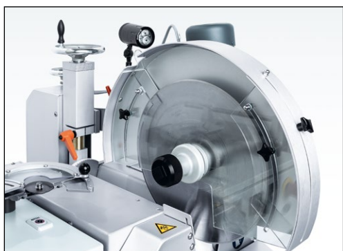
Figure 7-22 Bringing the circular knife grinding attachment into the grinding position
