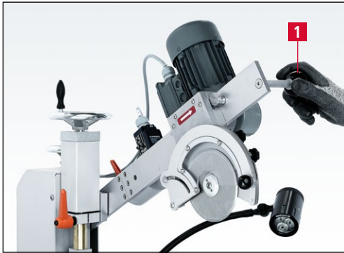
Figure 7-74 Bringing the grinding attachment into rest position
