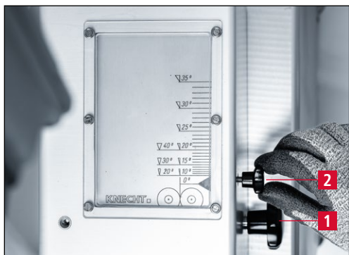
Figure 7-4 Setting the grinding angle
