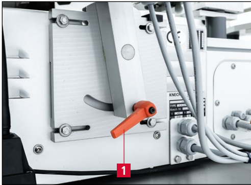
Figure 7-42 Loosening the clamping lever
