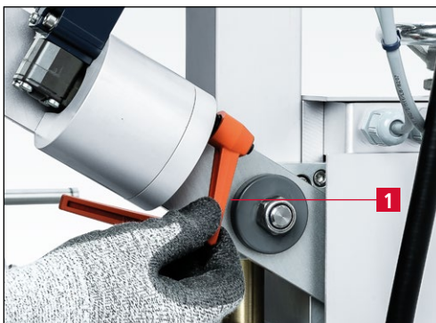
Figure 7-61 Loosening the "Mounting arm" clamping lever
