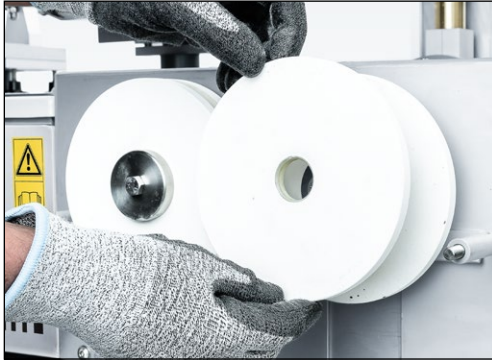
Figure 7-96 Removing grinding wheels and replacing with new ones
