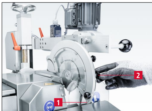
Figure 7-69 Setting the guard slide
