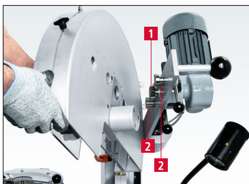
Figure 7-7 Mounting the circular knife holding fixture
