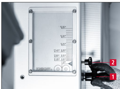
Figure 7-2 Locking the display arrow
