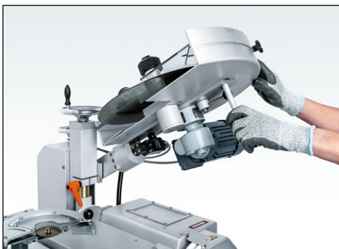
Figure 7-36 Bringing the circular knife grinding attachment into the clamping position
