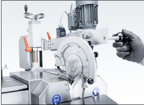
Figure 7-63 Bringing the circular knife grinding attachment into the grinding position
