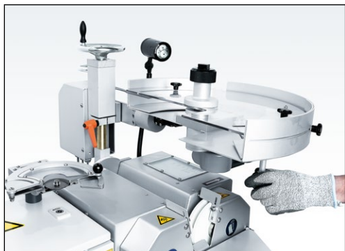
Figure 7-11 Circular knife grinding attachment in the clamping position
