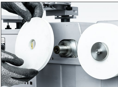
Figure 7-98 Removing grinding wheels and replacing with new ones
