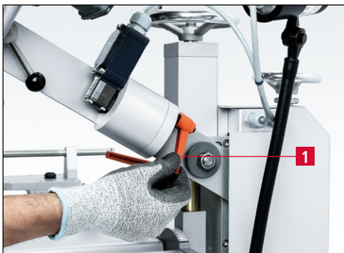
Figure 7-52 Loosening the "Mounting arm" clamping lever
