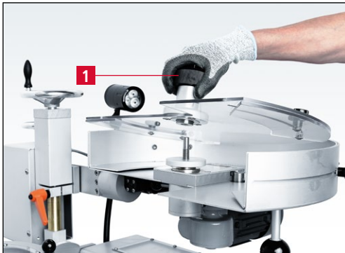
Figure 7-12 Removing clamping nut with the safety screen
