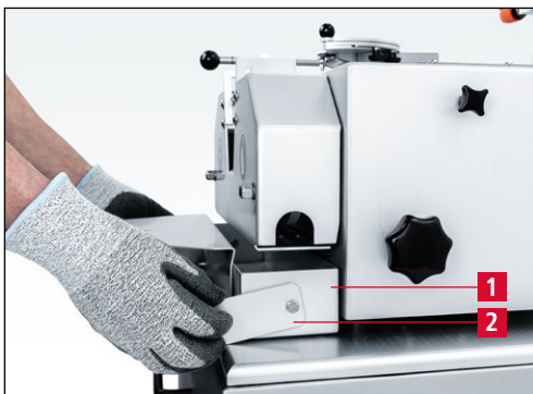
Figure 7-91 Removing the water tray
