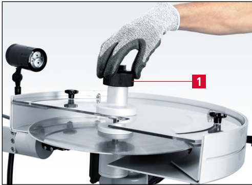
Figure 7-37 Unclamping the circular knife
