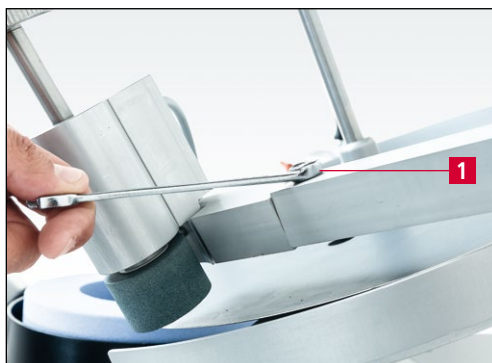
Figure 7-28 Swiveling the deburring arm
