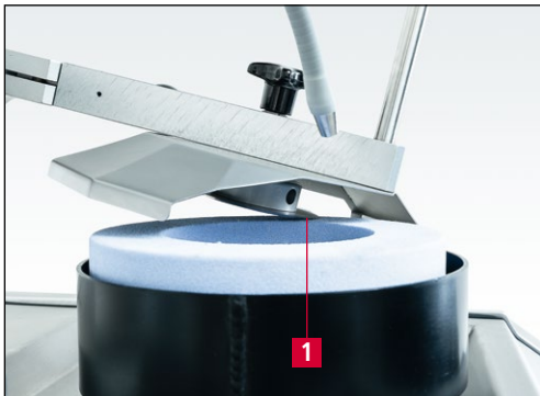
Figure 7-7 Positioning circular knives on the grinding wheel
