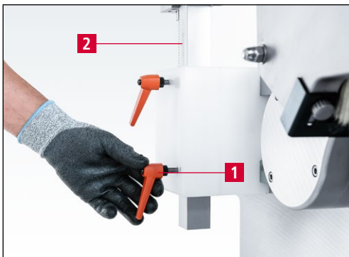
Figure 7-8 Positioning the circular knife on the grinding wheel
