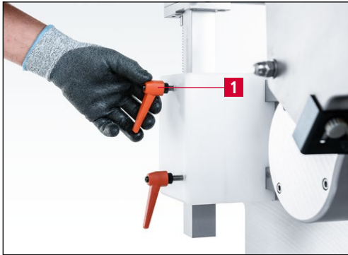
Figure 7-10 Loosening the clamping lever
