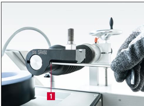
Figure 6-2 Loosening the set screws
