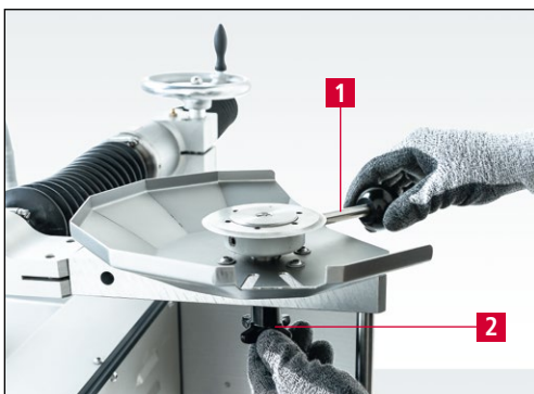
Figure 7-6 Clamping the circular knives
