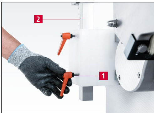
Figure 7-22 Adjusting the circular knife grinding attachment
