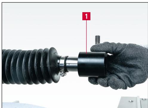
Figure 6-3 Removing the mounting head
